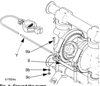
FIG. 1: Ground the pump
