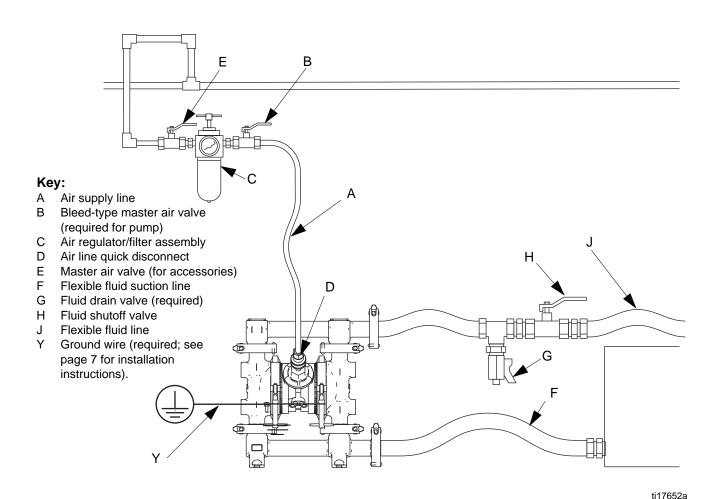
FIG. 2: Typical Floor-Mount Installation
