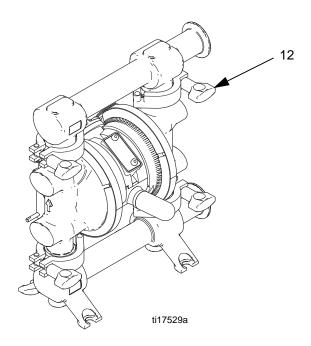
FIG. 3: Reverse the Manifolds
